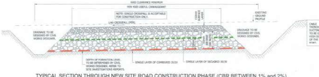
TYPICAL SECTION THROUGH NEW SITE ROAD CONSTRUCTION PHASE (CBR BETWEEN 1% and 2%) SCALE: 1:10
